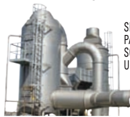
TWO STAGE HIGH INTENSITY SYSTEMS, VENTURI AND PACKED BED SCRUBBER IN SERIES
